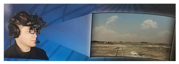
The EyeBox<sup>™</sup> solution consists of an SA-Photonics SA-92 helmet-mounted display with see-through 1920x1200 resolution per eye optics, a Polhemus Liberty head-tracking system, and a channel of the MetaVR Virtual Reality Scene Generator (VRSG) integrated with ZedaSoft's CBA® for Simulation framework.
