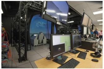
270 degree Immersive Displays Solutions (<u>http://www.immersivedisplayinc.com</u>) dome projection systems each running ten channels of MetaVR<sup>™</sup> (<u>www.metavr.com</u>) Virtual Reality Scene Generation (VRSG) visual scene rendering software. "We believe this integrated dual-dome solution developed by ZedaSoft continues to provide the best test platform and value for this very important life-saving technology." said GW Estep, president of ZedaSoft.
